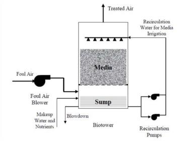
Figure 9-1. Simplified Schematic of a Biotower System
