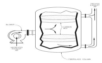
Figure 9-3. Schematic Dual Carbon Bed System
