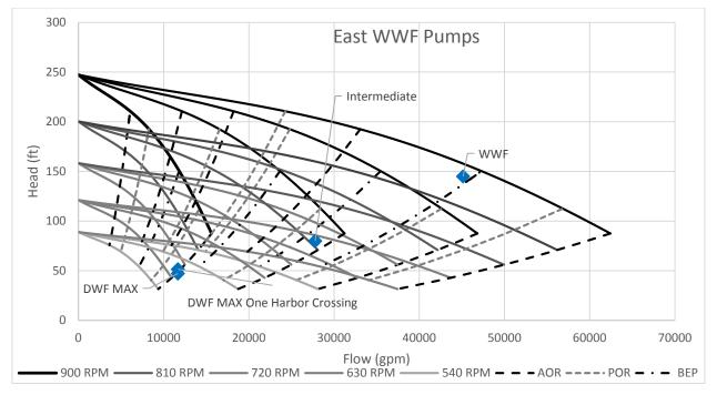
Figure 2-5. Wet weather pump and system curves
