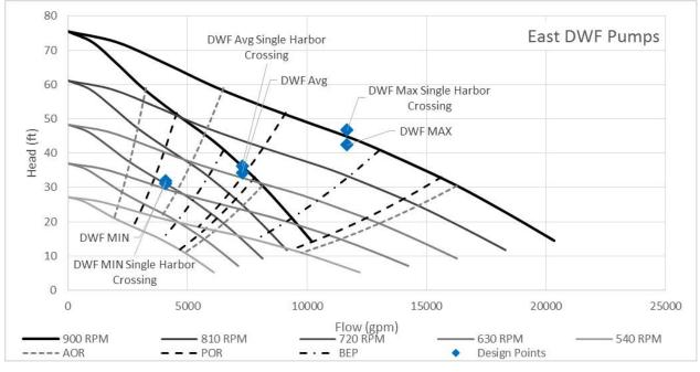
Figure 2-4. Dry Weather Pump and System Curves
