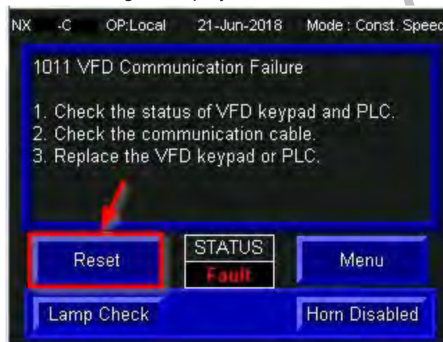
FAULT MESSAGE IN THE RESET SCREEN
